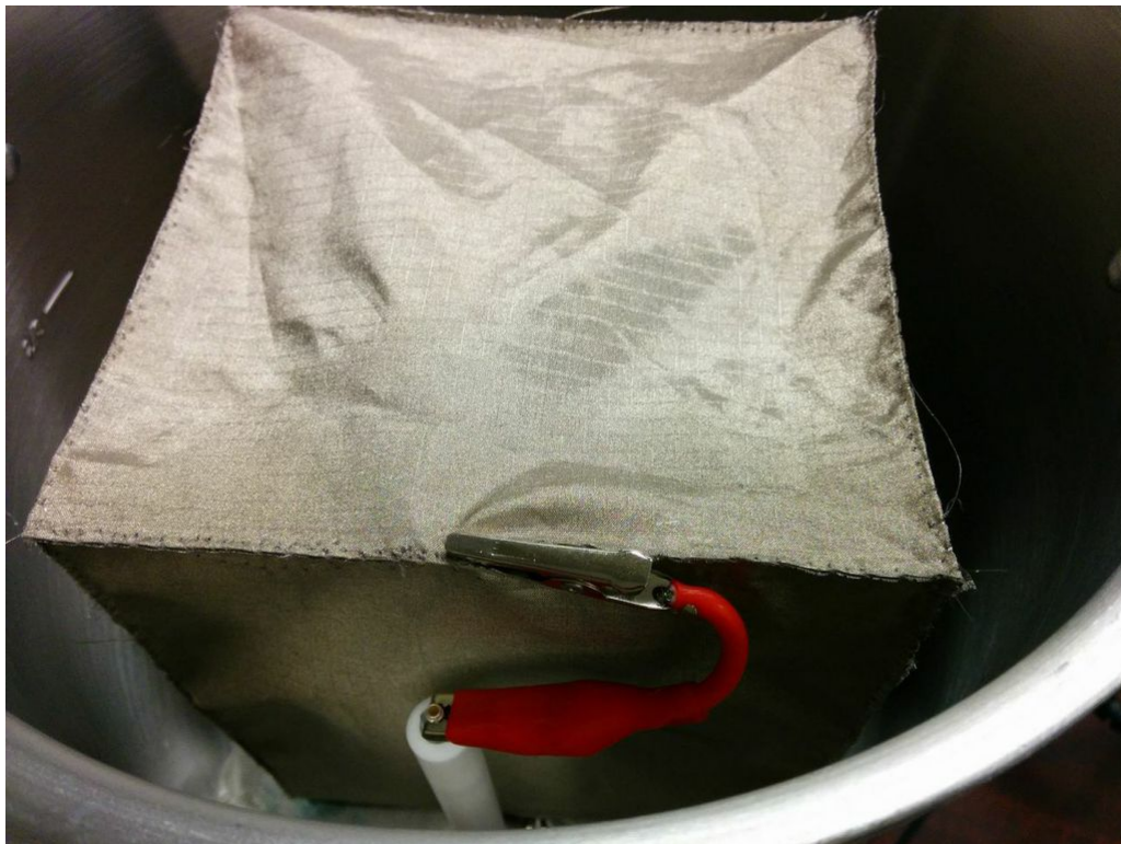
Figure 10 – Connection setup to transfer voltage from the high voltage lead to the fabric
