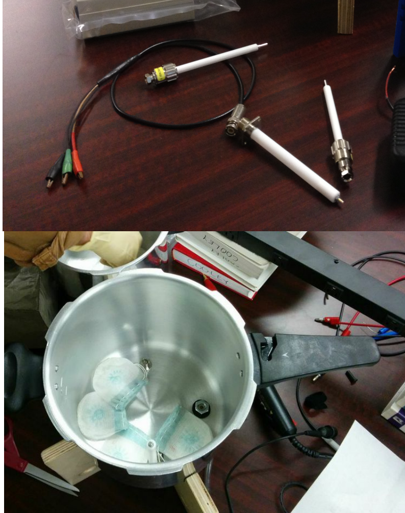
Figure 6 – High voltage connector within the pressure cooker setup
