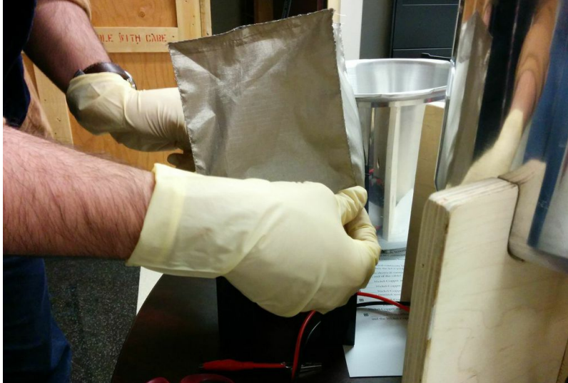
Figure 9 – NiCu fabric being placed over the 3D-printed copper holder
