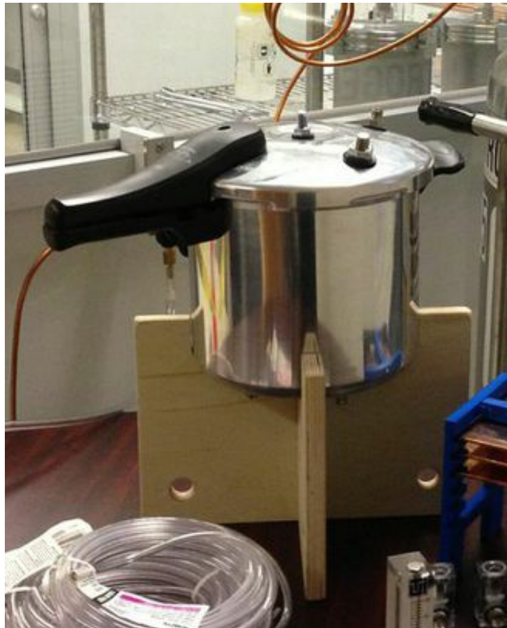
Figure 5 – Pressure Cooker setup with modifications for input and output
