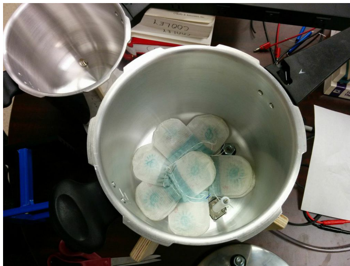
Figure 3 – Camping lantern mantles in position for experiment within the pressure cooker
